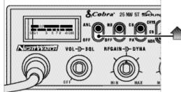
• When *switched* to ANL the Automatic Noise Limiter is activated. This helps reduce noise created by the vehicle's electronics.
