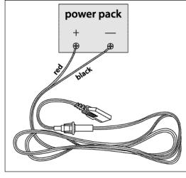
Simply connect the red (+) and black (-) leads of the transceiver to the corresponding terminals of the power pack.
