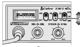
When *switched* to NB position the RF Noise Blanker is activated, providing increased noise filtration. When switched to OFF position Noise Blanking Filtration will be turned off.
