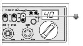
• Switch to R NOR to select desired channel.
