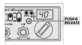
● Push and release the ST button. Red LED is illuminated when SoundTracker<sup>™</sup> is turned on.
