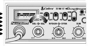
To achieve the Desired Squelch Setting (DSS), turn the Squelch control counterclockwise until you hear noise. Now turn the control clockwise just until the noise stops. This is the DSS setting.
